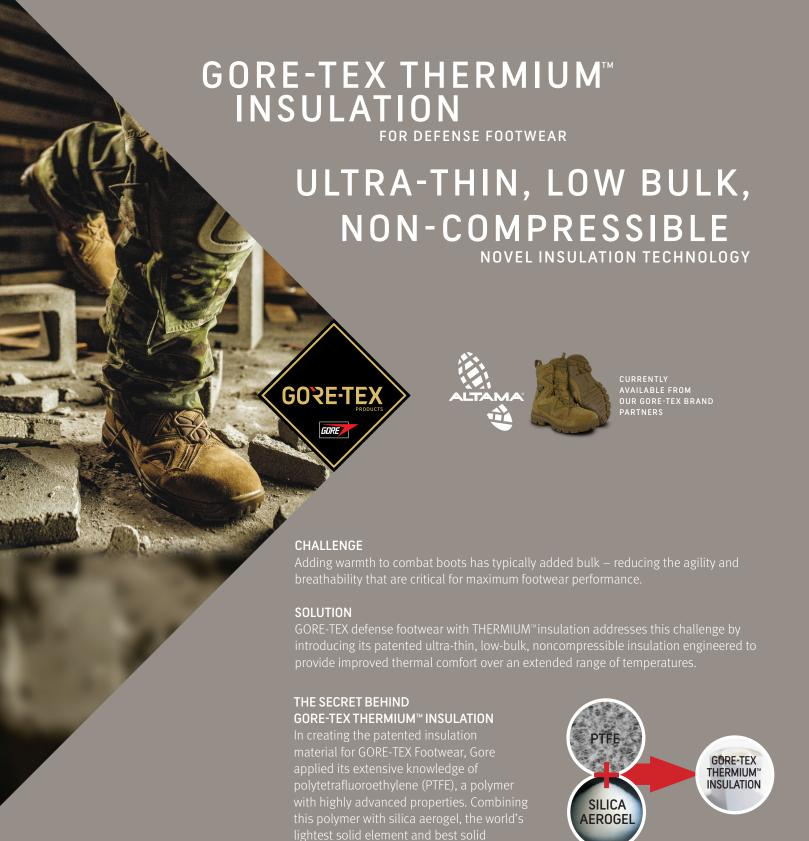
Developed by NASA for such uses as helping shuttles re-enter the atmosphere, aerogel provides unparalleled insulation. On its own, the aerogel is stiff and difficult to maneuver. The addition of PTFE creates a flexible and compression-resistant insulator, with a thickness of about 1.7 mm. The material can be cut and treated like leather and applied to combat boots in a way that retains boot breathability and agile performance
