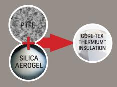
Developed by NASA for such uses as helping shuttles re-enter the atmosphere, aerogel provides unparalleled insulation. On its own, the aerogel is stiff and difficult to maneuver. The addition of PTFE creates a flexible and compression-resistant insulator, with a thickness of about 1.7 mm. The material can be cut and treated like leather and applied to combat boots in a way that retains boot breathability and agile performance.
