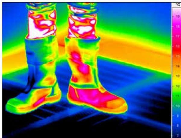
Conductive heat loss of a GORE-TEX EXTRAGUARD safety footwear (right shoe) is considerably less than that of an identical leather version.
