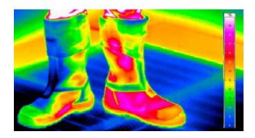
Conductive heat loss of a wet GORE-TEX EXTRAGUARD safety footwear (right shoe) is considerably less than that of an identical leather version.
