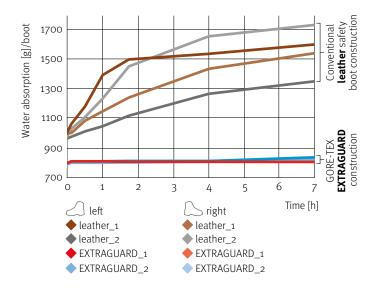
Compared with conventional safety footwear, GORE-TEX EXTRAGUARD footwear has very low water absorption.
