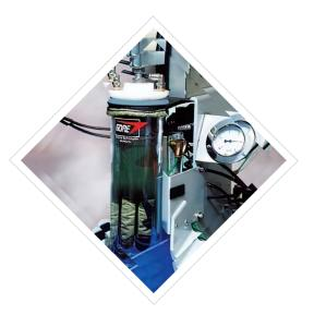
The GORE Whole Glove Leak Tester is the first practical leak detector for gloves. The whole glove leak tester fills gloves made with GORE-TEX CROSSTECH<sup>®</sup> Glove Inserts with pressurized air. If the pressurized air passes through even a tiny pinhole, bubbles will appear below in a water trough.
