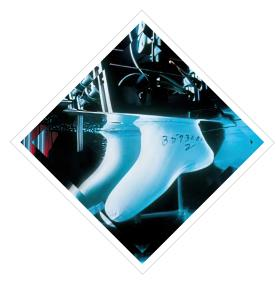
Every bootie made out of GORE-TEX CROSSTECH® Footwear Fabric must pass a waterproofness test before being used in leather footwear. The bootie is filled with air and then submerged in water to check for leaks.
