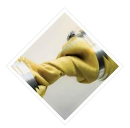
Testing using the Gelbo Flex Tester allowed Gore to show that GORE-TEX CROSSTECH<sup>®</sup> 3-Layer Moisture Barrier retained its liquid penetration resistance after repeated flexing and twisting.
