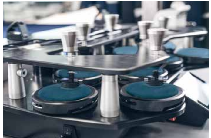
High abrasion resistance in Martindale testing
