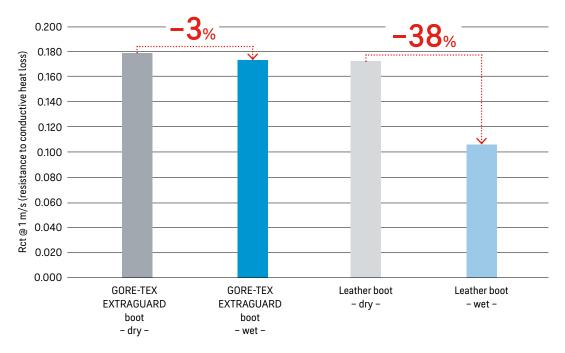
Identical boots were compared when dry and when wet. The potential heat loss of wet leather boots is significantly higher than that of wet GORE-TEX EXTRAGUARD boots.
