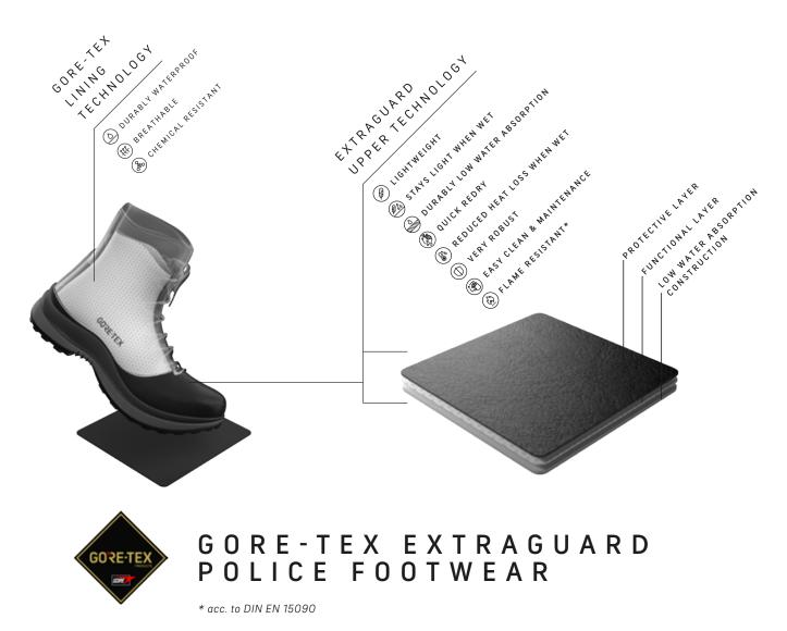
3-layer technically engineered upper construction - seam-sealed with GORE SEAM® Tape - and GORE-TEX lining (bootie construction).
