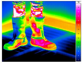
Conductive heat loss of a GORE-TEX EXTRAGUARD boot is considerably less than that of an identical leather version.
