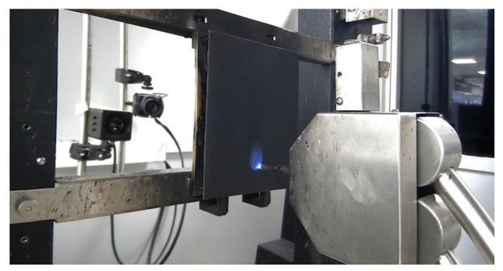
GORE-TEX EXTRAGUARD upper material does not inflame when exposed to a Bunsen burner for 10 seconds.
