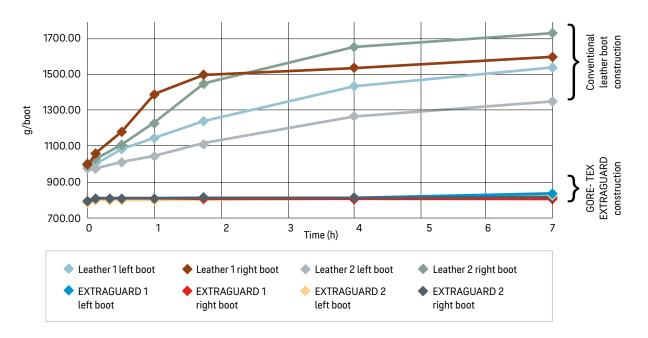
Compared with conventional boots, GORE-TEX EXTRAGUARD boots have very low water absorption, confirmed by the water bucket test.
