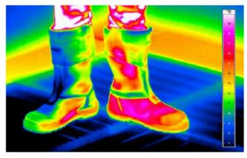
Conductive heat loss of a wet GORE-TEX EXTRAGUARD boot is considerably less than that of an identical leather version.
