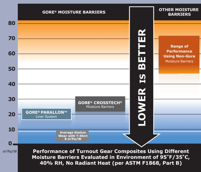
When tested using the ASTM F1868, Part B method, GORE® barrier technologies created less resistance to evaporative sweat transfer, enabling higher breathability when evaluated in the same outer shell and thermal liner combinations.
