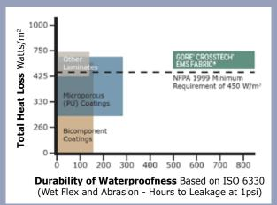
\*Data derived from typical Gore laminate performance. Note: An Rct value of all materials has been assumed to be .067°Cm²/W in the THL calculation. A lining Ret of 20 ( $m^2$ mbar/W  $\times$  103) has been added to all "2-layer" garments.
