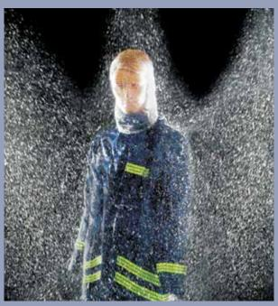
The NFPA 1999 Liquid Integrity Test evaluates a garment's design, construction quality, and seam sealing for waterproof integrity.
