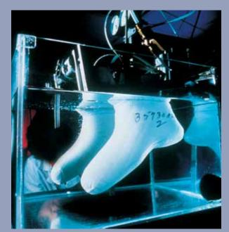
Every bootie made out of GORE® CROSSTECH® Footwear Fabric must pass a waterproofness test before being used in leather footwear. The bootie is filled with air and then submerged in water to check for leaks.
