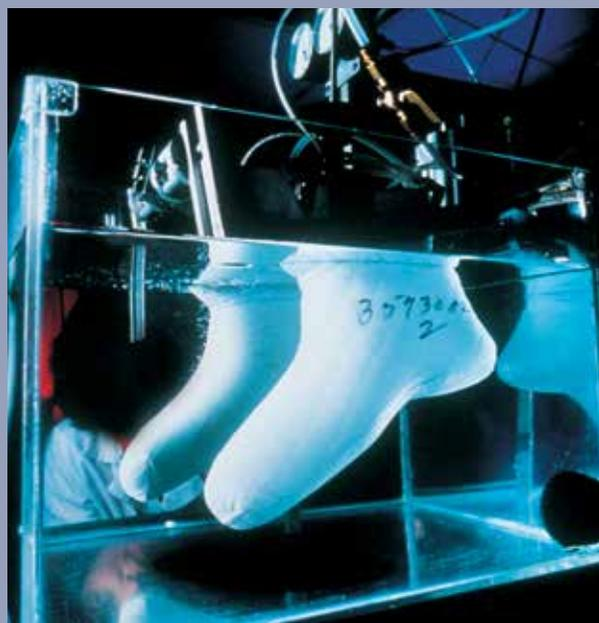
Every bootie made out of GORE® CROSSTECH® Footwear Fabric must pass a waterproofness test before being used in leather footwear. The bootie is filled with air and then submerged in water to check for leaks.
