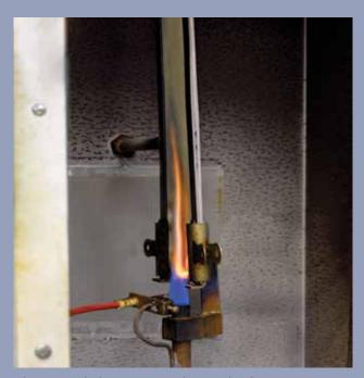
The Vertical Flame Test evaluates the flame resistance of GORE® CROSSTECH® S/R Fabric. It exposes the material to a flame for 12 seconds and monitors burning behavior when the flame is removed. This test measures burn time after the flame is removed, char length, and the ability to withstand melting and dripping.
